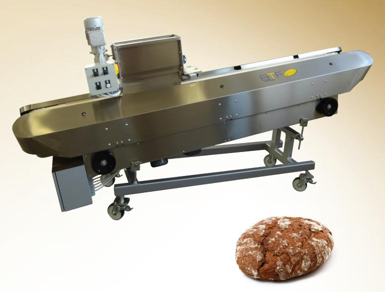
**Belt rounder** consists of two contrarotating belts from nonstick material with possible regulation of working width. Easy and fast adjustment for any round product with high weight range. Belt rounders are the most convenient for rounding rye and wheat-rye type of dough.
